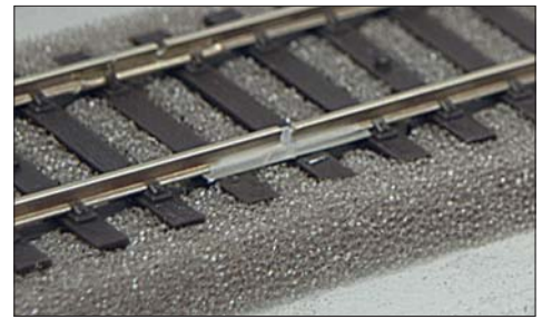
Above: note the nylon insulating rail joiner. This will be a section of track where the feed wires can be switched on or off to activate or isolate the section.
