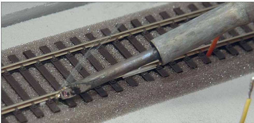
Above: the wire is tinned with flux and solder to ensure a reliable electrical contact with the rail.
