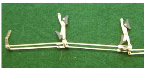
Above: the underside of the finished tender showing the split axles in situ. This is what to aim for.
