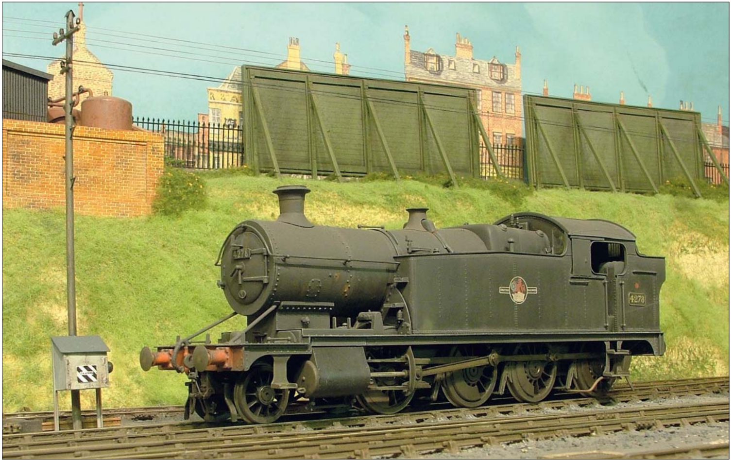
Above: ex-GWR 42xx 4278 on shed after bringing in a coal train from South Wales. It is a David Andrews kit with RG7 motor and gearbox, and Slater's wheels. Built by Chris's son.
