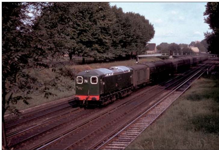
Above: Bulleid/Raworth Co-Co electric No.20002 hums its way south through Wandsworth Common with a Victoria-Newhaven boat train on 20 September 1964, four years before retirement. The three SR electric locos were regulars on this duty.
