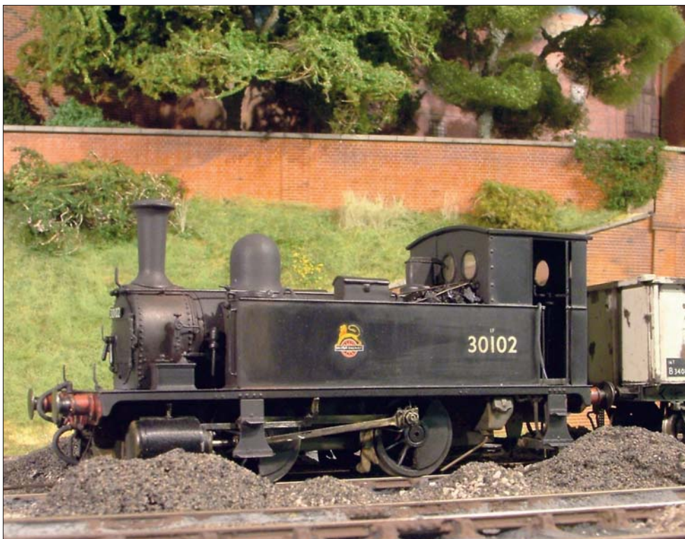
Below right: Adams B4 30102 was built from an ABS kit with an ABC gearbox and Maxon motor, sprung hornblocks and split-axle current collection.
