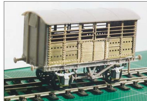
Above: the top of the solebar is level in reality! The Ratio plastic is soft, and tends to roughen up even when cut with a fine razor saw.
