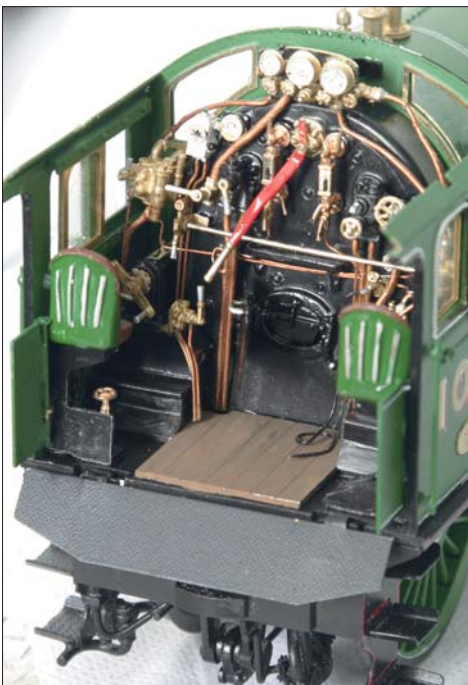
The cab interior, partly complete (above) and finished (below). The reverser handle can be turned, just as on the prototype, and the fire-hole door can be opened.
