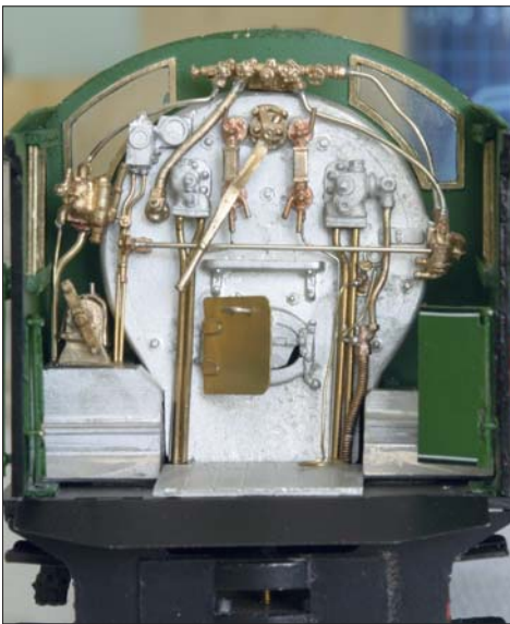
The cab interior, partly complete (above) and finished (below). The reverser handle can be turned, just as on the prototype, and the fire-hole door can be opened.
